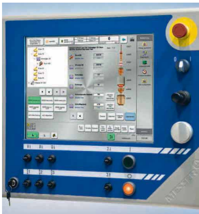
The Messer cutting system is particularly easy to operate with the Global Control CNC. An automatic back-up program saves the database contents to a server
