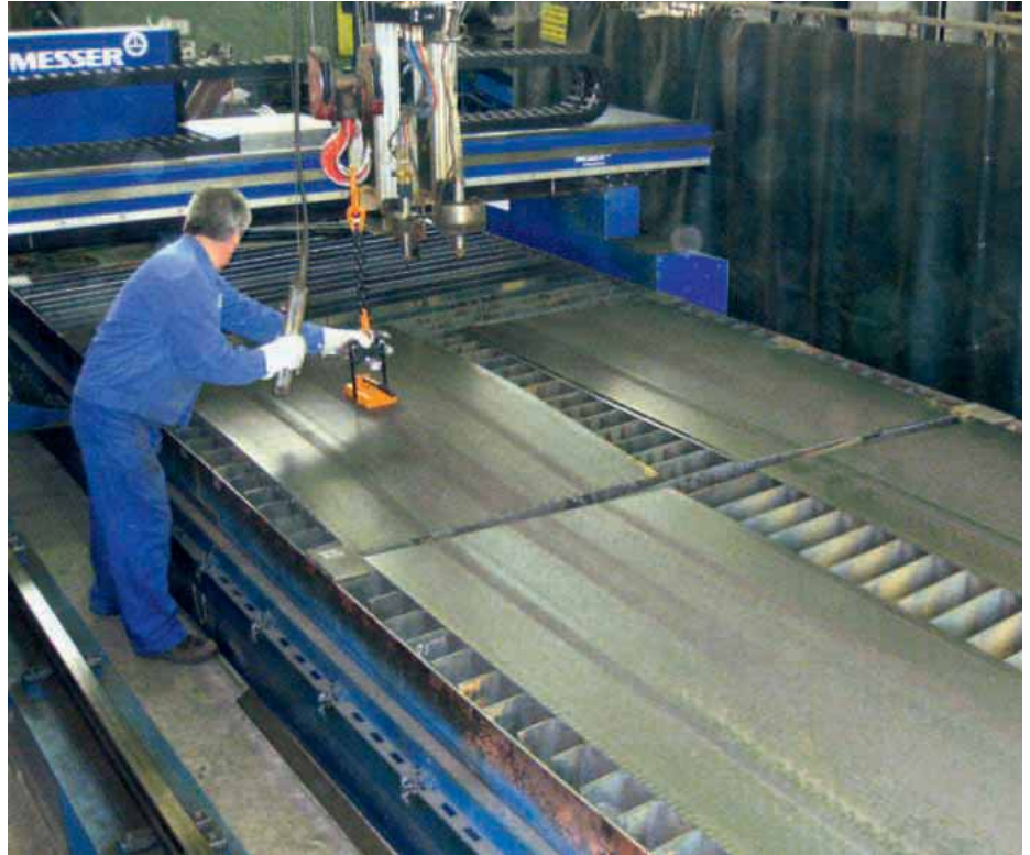
Efficient production cycles at Spinner Stahlbau GmbH: The "Joblist" function on the Messer Global Control CNC makes it possible to load four plates at a time to cut them then one after the other with the Messer MultiTherm
