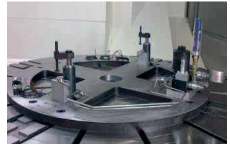
One of the Roemheld setups used by the MTC to investigate the effects of centrifugal force on hydraulic workholding
