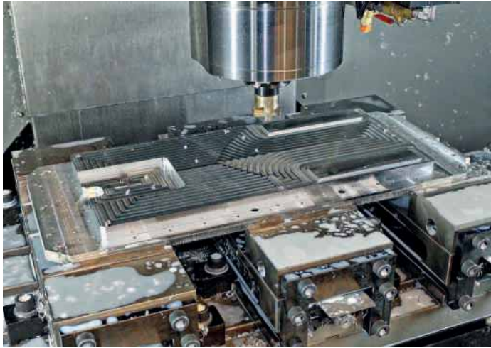
A 6082 aluminium test base plate for a military aircraft being machined on the VMX30i
