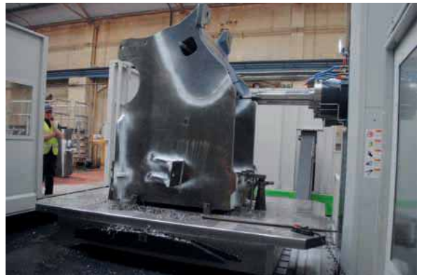
The Doosan DBC160 installed at Terex is a powerful, rigidly-built horizontal boring machine capable of machining large, heavy and awkward-shaped workpieces
