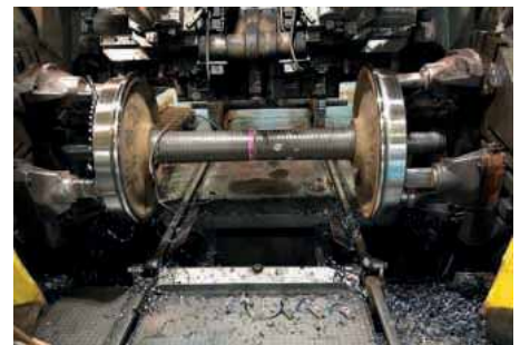
The same wheel profiling application now with chip control, using Dormer Pramet's modified LNMT insert
