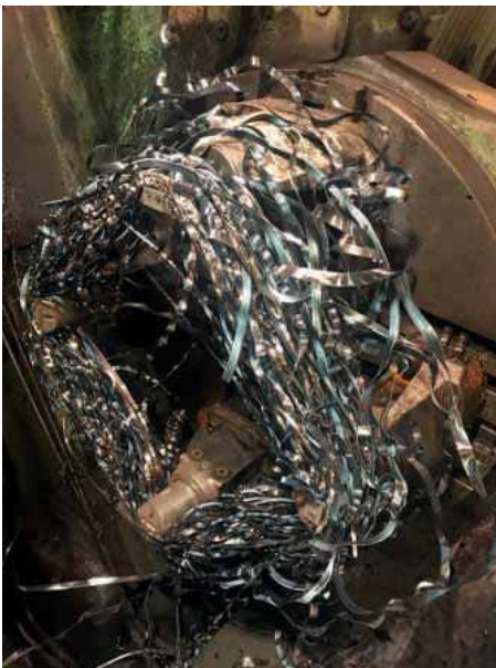
A wheel profiling application with no chip control
