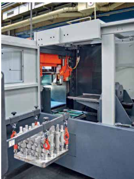
A batch of 3D printed titanium shafts for locking aircraft doors being delivered by forklift truck to the KASTOwin amc
