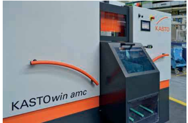
Airbus Helicopters uses a KASTOwin amc bandsaw to separate additively manufactured components from the base plate
