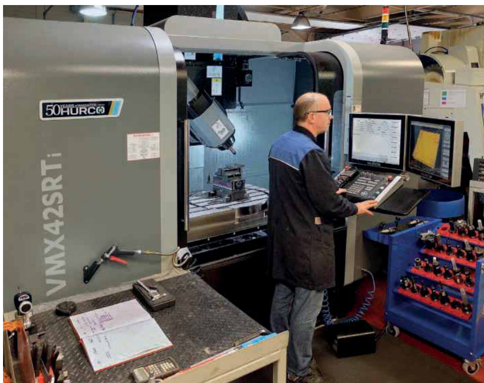
One of the pair of Hurco VMX42SRTi 5-axis machining centres installed at the Livingston factory of Almond Engineering
