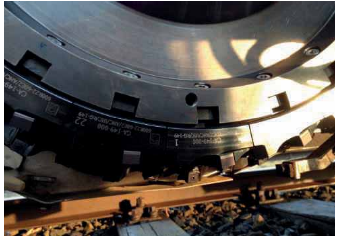
Dynamic rail milling application in operation using the Dormer Pramet cutter and inserts
