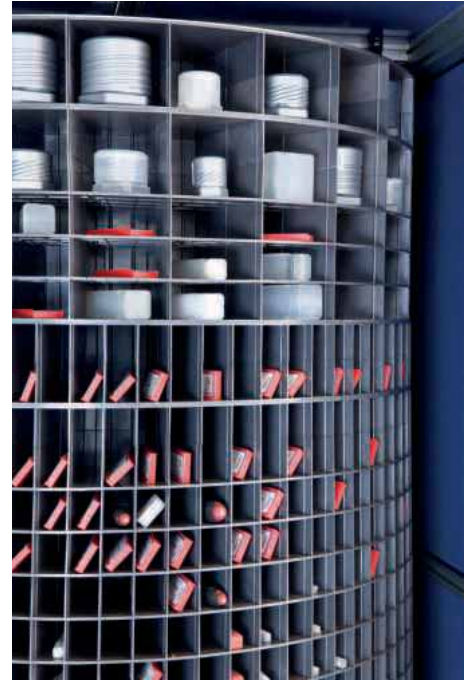
The carousel system of the ARNO StoreManagerPRO offers up to 2,160 compartments
