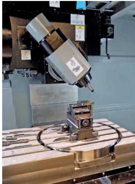
Working area of the Hurco VMX42SRTi 5-axis machine showing the B-axis spindle and C-axis flush rotary table
