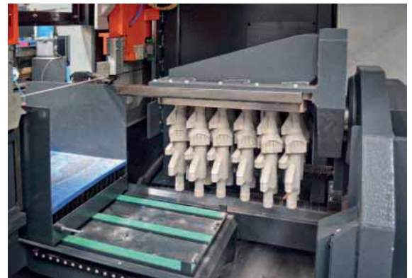
Bandsawing is performed in the KASTOwin amc with the workpieces inverted to prevent damage to the expensive 3D printed parts after their separation from the base plate
