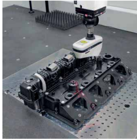
A plastic injection moulded rocker cover from JCB Power Systems' R&D department in Derby being inspected in Chapeltown using the cross scanner
