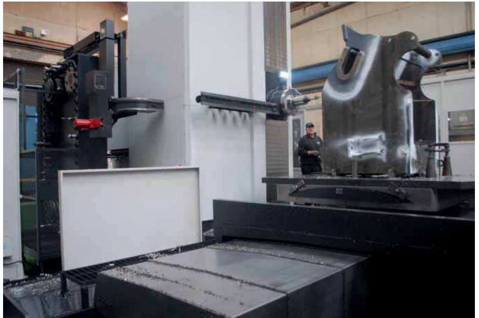
The Doosan DBC160 installed at Terex is a powerful, rigidly-built horizontal boring machine capable of machining large, heavy and awkward-shaped workpieces
