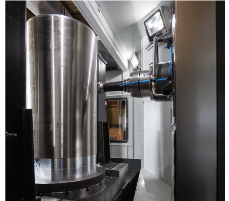
The WNT 100 mm facemills and other tooling that will reduce this 316 stainless steel billet from 3 tonnes to 0.5 tonnes over many 100s of hours of machining cycle
