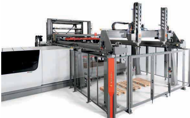
Modular automation for laser cutting: with the BySort upgrade, unloading and sorting with the ByTrans Cross becomes even more versatile
