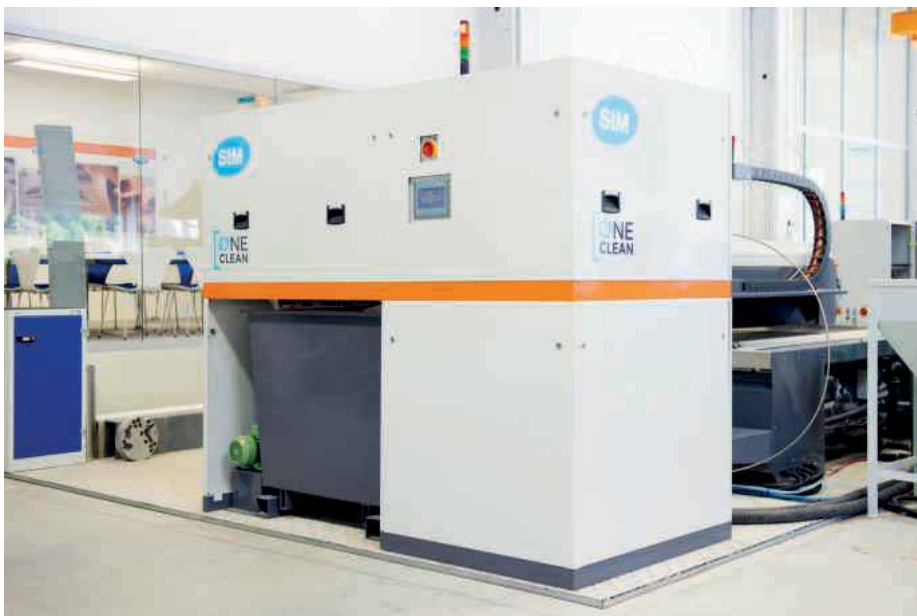
The OneClean modular system for fully automatic recycling of water and abrasive sand
