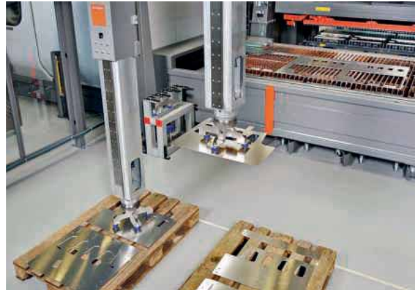
Increased processing quality: automated unloading of cut parts using BySort ensures safe, fast and accurate material handling
