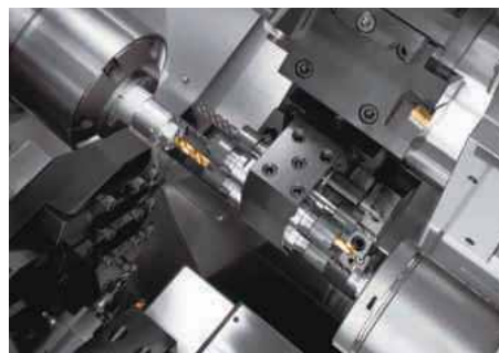
Tooling zone of Miyano BNA-42GTyLFV showing three tool simultaneous cutting
