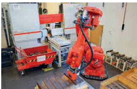
A robot places cut sections on one of four pallets
