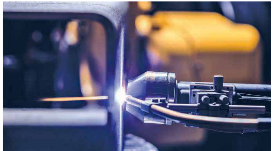
The ArcTig welding process from Fronius achieves high welding speeds and outstanding weld seam quality
