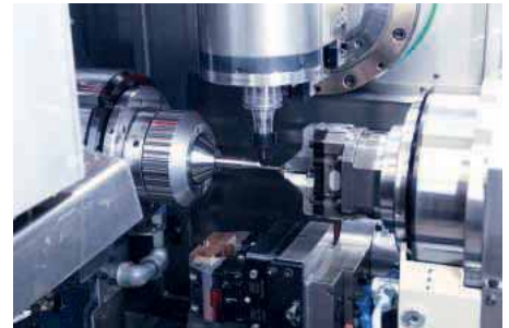
The working area of the seven-axis Bumotec s191H linear CNC turn-mill centre that was demonstrated at the AMRC with Boeing Centre
