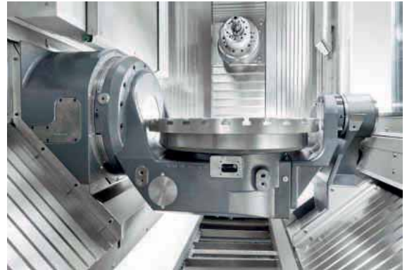
The work area of the new Heller HF 3500 horizontal-spindle, 5-axis machining centre that will make its UK debut at MACH 2018
