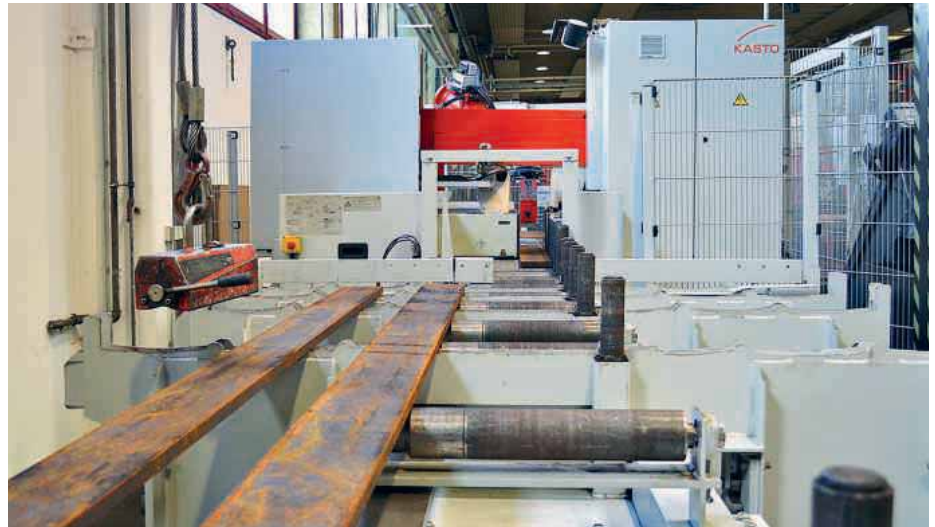
A magazine with space for four bars up to 3,500 mm long supplies the KASTOtec FC 4 bandsaw
