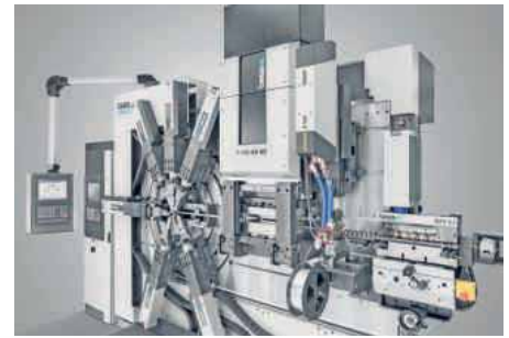
Bihler B 20K high-performance welding control system with servo-controlled GRM-NC stamping and forming machine and Quickchange contact welding module
