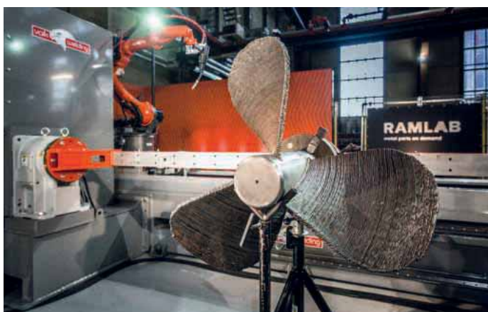
The world's first class-approved 3D printed ship's propeller Photo Credit: Image courtesy of RAMLAB
