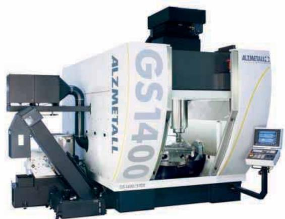
revs/min motor with 500 Nm of torque with tool magazine options between 33 and 250 pockets. Tools up to 125 mm dia, 250 mm with adjacent pockets left empty, can be exchanged in seven seconds chip-to-chip.
