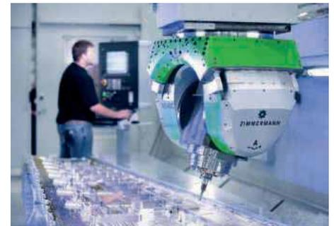
Removal of sharp edges with a milling cutter eliminates possible stress points, takes away material that could otherwise detach and cause blockage or wear, improves a component's appearance and promotes safe handling. Titanium aerospace components can be profiled so that edge radii are within  $\pm 25$  microns and surface finish is better than Ra 0.8.
