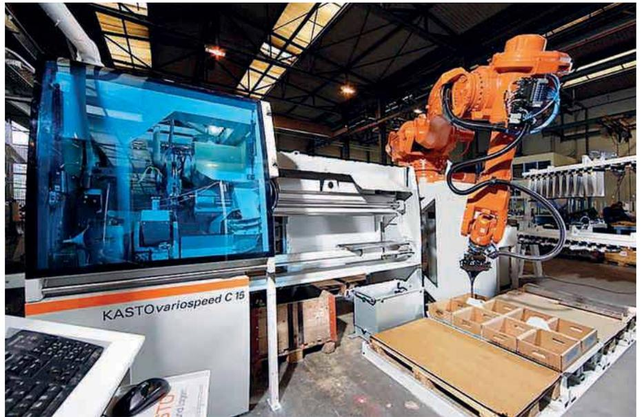
sawing machine can run attended, with the control system holding all parameters of a job including material diameter, band speed, rate of downfeed, cut length and number of parts.
