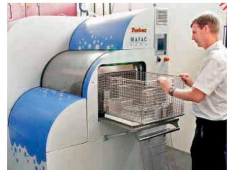
For processing larger parts such as casings, landing gear components as well as aerostructures, Turbex offers the ACV range of front-loading, spray washing and rinsing models. They are particularly popular for degreasing and precision cleaning prior to NDT. Standard sizes range from one to three metres in diameter, although larger machine sizes are available.
