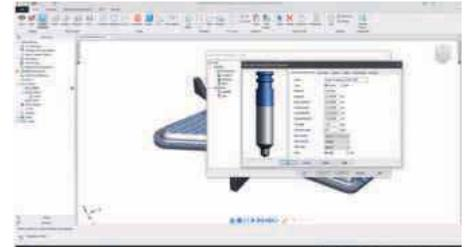
introduction of additional parameter controls for centre drills.
