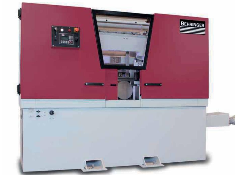
of vibration-damping grey cast iron and double band wheel bearings work together to ensure quiet running and cutting precision. Trials confirmed a 30 percent longer service life of bandsaw blades alongside visibly better cut surface quality. The slight inclination of the band wheels helps prolong the life of bandsaw blades by reducing fatigue due to cyclical bending.
