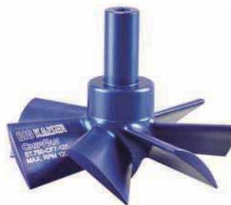
remaining chips or coolant, thus performing two cleaning operations in a single step. Ideally, the Chip Fan should be programmed into the machining cycle to minimise spindle downtime and maximise operator efficiency. Safety is also improved as all the swarf and coolant is neatly contained within the machining enclosure and kept off the shop floor.
