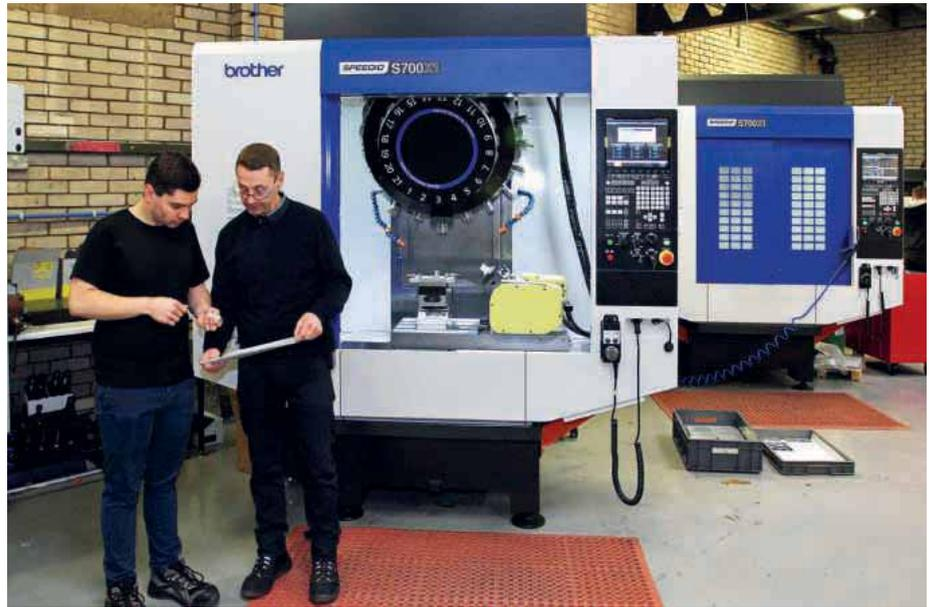
Since the machine was installed, CTPE has gone a step further by optimising the program to machine six parts on the table with 14 tools and adopting new types of cutters. The effect has been to reduce the cycle time per part further to just 30 percent of the original.
