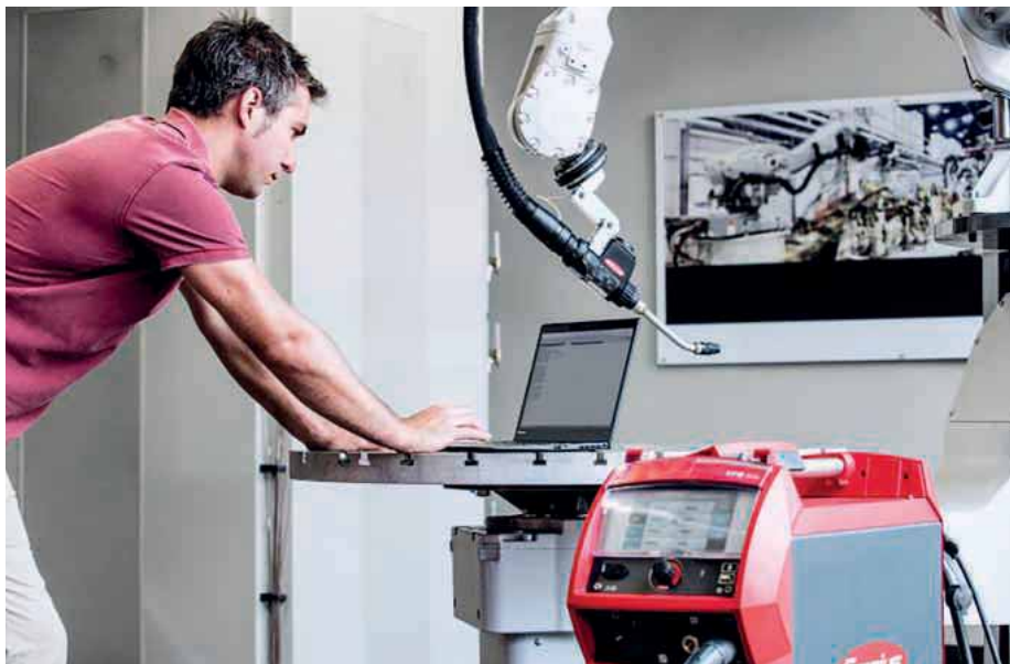
Thanks to function packages the welder can use several processes on the TPS/i such as LSC (Low Spatter Control), PMC (Pulse Multi Control) as well as CMT (Cold Metal Transfer) on one device
