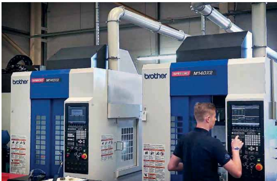
The two M140X2 5-axis, 30-taper machining centres on the shop floor at Plalite's Sittingbourne factory. They are fitted with Brother's latest, high speed C-00 control system
