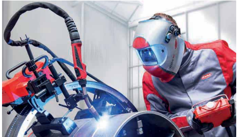
The FlexTrack 45 Pro offers a constant travel speed for optimal, reproducible welding results
