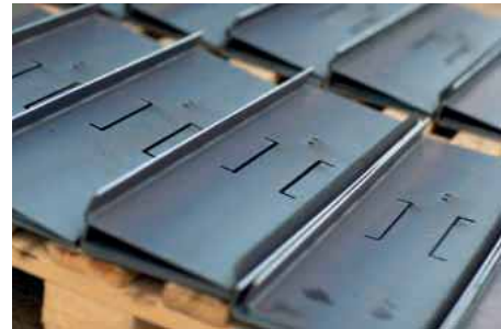
BSK components cut on the Kerf RUR machine
