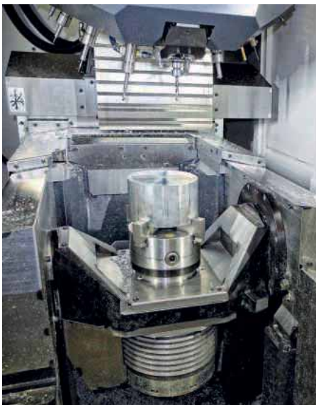
Close-up of the aluminium fixture about to be produced. The machine's working envelope is 200 x 440 x 305 mm and the A-axis trunnion is tilted from +120 to -30 degrees by a backlash-free roller drive
