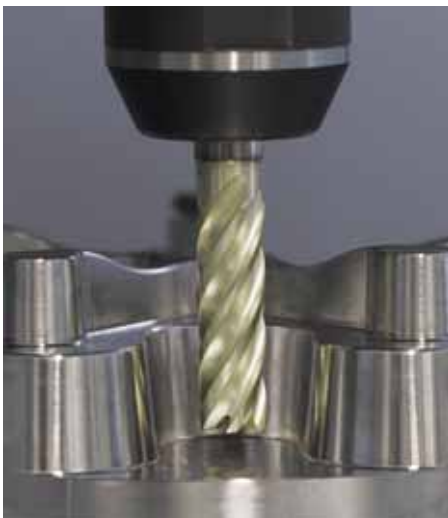
Walter's MD133 Supreme is ideal for high-dynamic milling applications
