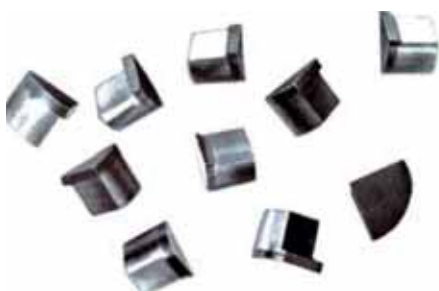
Unmachined synthetic cutting inserts - developmental status as of 1973. The shown segments with 60° and 90° angles were mechanically cut out of PCD blanks (of approx \varnothing 3.4 mm) with diamond cutting wheels
