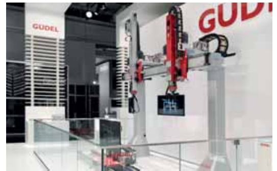
Güdel's new telescopic axis design requires significantly less headroom but delivers the same payload capacity of a standard axis
