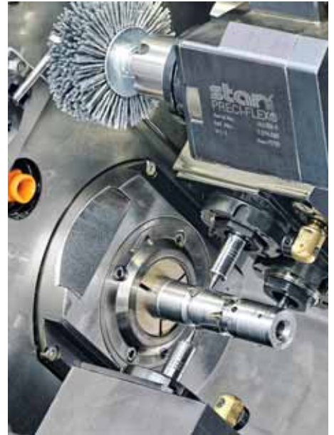
The precision toolholders can clamp all tool shanks with h6 tolerances and diameters of at least 1.0 mm
