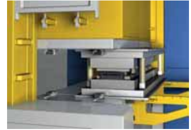
Typical wedge clamp positioning on a power press
