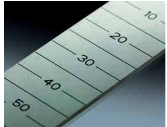
High contrast marking on metals using picosecond laser pulses extends viewing angle and improves quality especially for medical device applications
