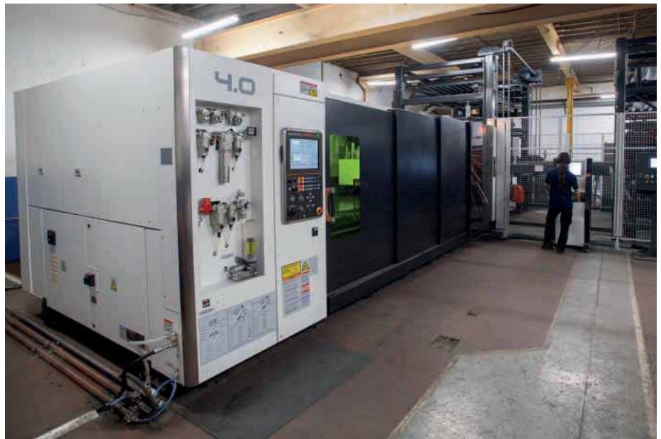
The OPTIPLEX NEXUS 3015 Fiber 4kW laser machine with bespoke 10-shelf automation towers, at CSM's Swansea Mill works
