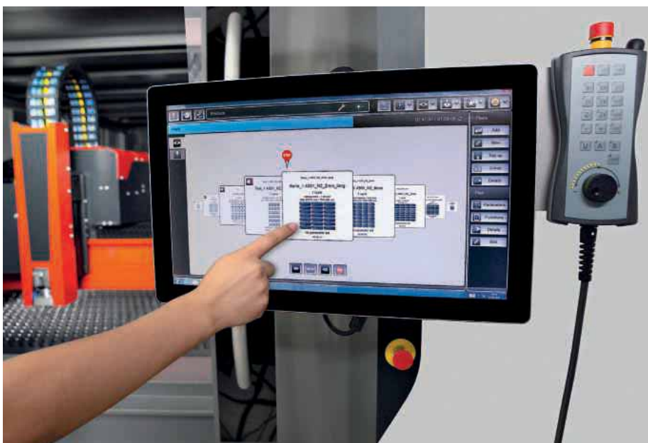
The cutting process is controlled via a 22-inch touch screen
