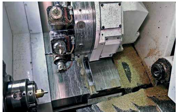
The machining area of the Genos L3000e. The lower milling cutter in the 40 VDI turret is 50 mm diameter
