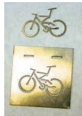
Legend Laser's new SRC-610 system can cut complex sheet metal parts to plus/minus 10 microns accuracy
