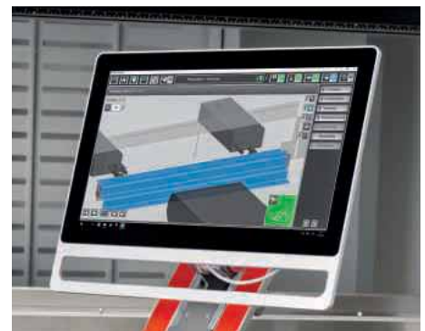
Operation is simple using a touch screen and ByVision Bending software
