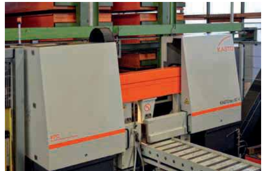
The high-performance KASTOtec SC 4 bandsaw purchased in 2016 is designed to process larger diameter stock, in particular solid and difficult-to-cut materials
