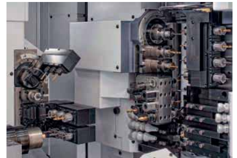
The CNC sliding-headstock turn-mill centre has proved to be the ideal machine tool platform on which to produce ventilator parts. Pictured is the Citizen Cincom D25-VIII LVF
