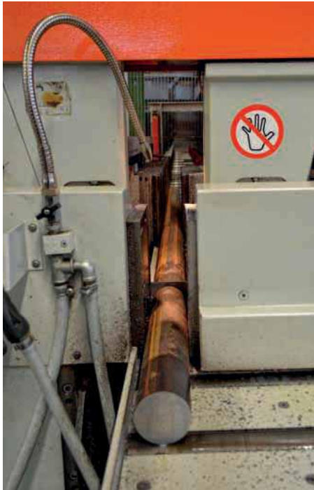
The saw features a cutting range of 430 mm and can operate with HSS or carbide bandsaw blades
