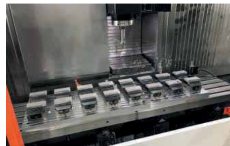
COVID-19 ventilator parts ready for machining
