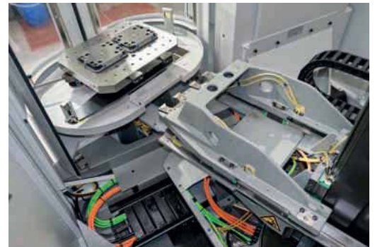
A view of the robotic transfer arm that moves pallets automatically between the workpiece load/unload station in the background, their storage positions and the Hermle C 400's working area
