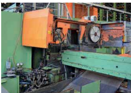
The original KASTOhba bandsaw was still mechanically sound, so in 2019 it was refurbished along with the existing KASTO storage system for steel bar and tube
