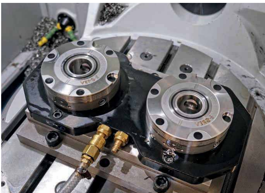
A pneumatically actuated SCHUNK zero-point fixturing system ensures speedy changeover between operations on the Spinner
