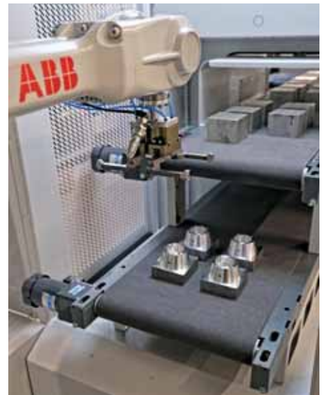
The 6-axis ABB robot with a double gripper for handling raw material from the upper conveyor into the machining centre and finished parts onto the lower conveyor after machining. Both conveyors can be up to 5 m long
