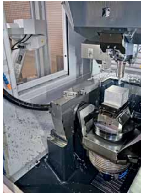
The working area of the Speedio M300X3 mill-turn centre showing the trunnion arrangement, torque table for turning operations and the robot positioned to the side
