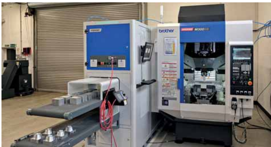
The Speedio / Feedio demonstration cell in Whitehouse Machine Tools' Kenilworth showroom. Accessibility to the machine from the front is maintained, as the automation unit is positioned to the side, a configuration that allows two machining centres to be served
