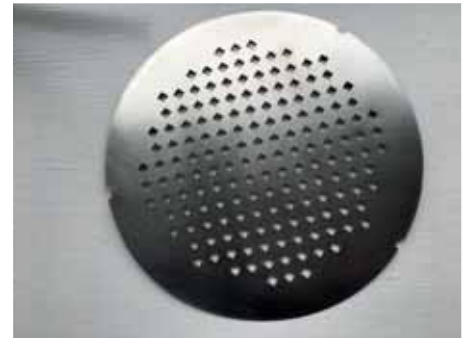
A precision exposure mask created by erosion cutting
