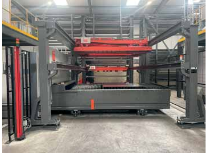
Loading system and Bystar laser bed
