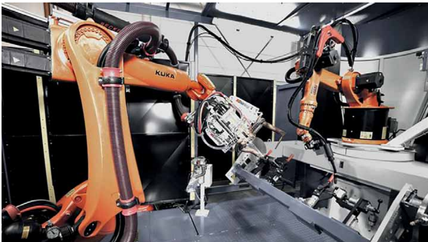
The KR 6-2 (on the right) performs the arc welding while the KR 210 guides the servo-pneumatic robotic gun
