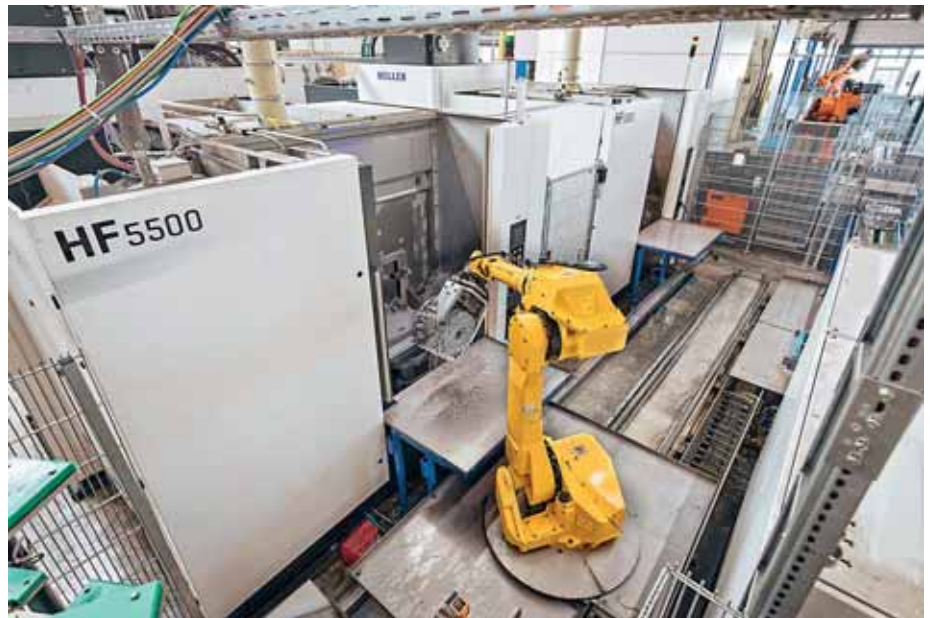
The production line at the Stöferle Automotive factory in Laupheim into which two second-generation Heller 5-axis HF 5500 HMCs have been integrated
