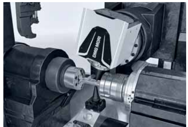
Working area of the NTX 500, showing the upper B-axis tool spindle and lower turret
