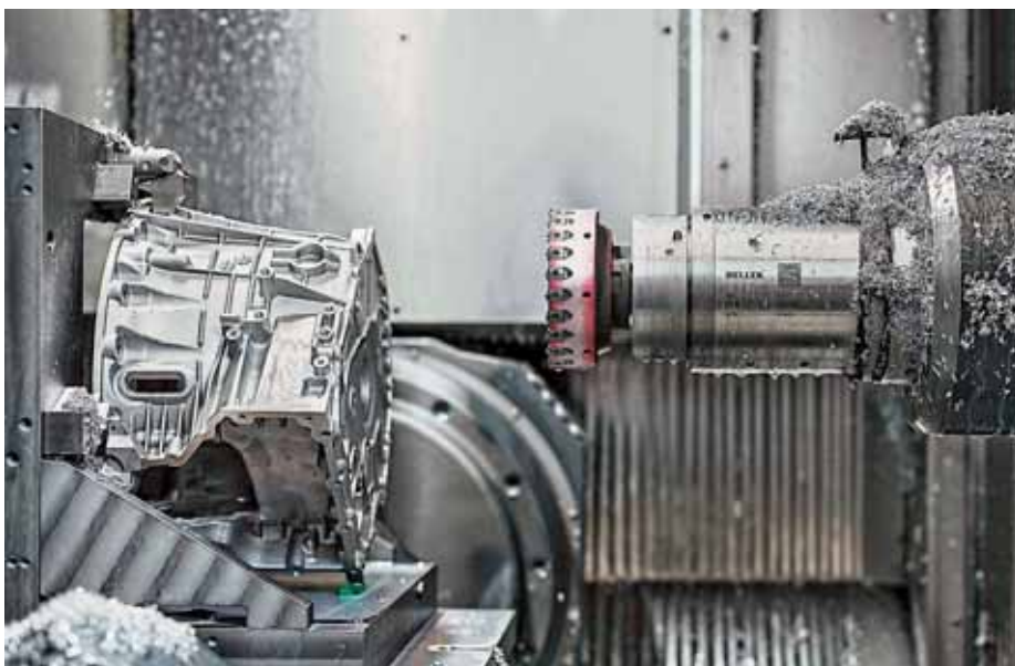
A drive motor housing for a hybrid vehicle being machined in one of the Heller HF 5500s
