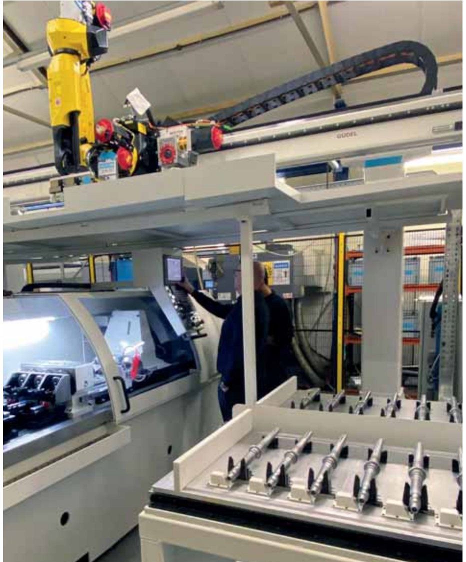
A space-saving gantry rail with a FANUC M-20iD/25 6-axis robot transfers parts between the three-machine cell
