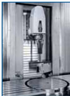
*Tool change now takes place safely behind the work table, avoiding interference with fixtured workpieces and contributing to thermal stability*
