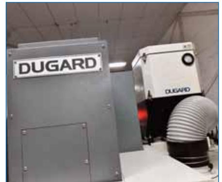
*The new Dugard filtration system on the Dugard 550 machine*
