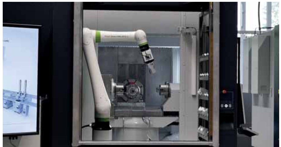
A FANUC Cobot loading a Starrag machine at the Starrag Tech Days event.
