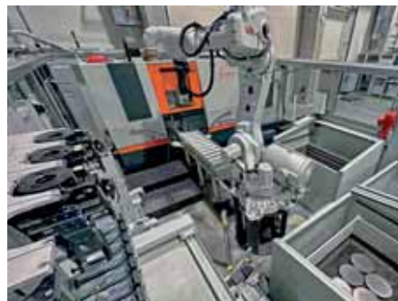
At SEW, the KASTOtec SC 4 automatic bandsaw cuts material up to 260 mm in diameter, although the machine has a capacity of 430 mm.
