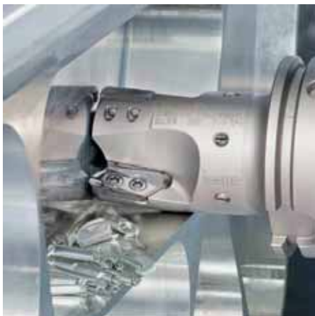
Fig. 2: Indexable milling cutters for machining aluminum at extremely high cutting speeds are specifically engineered to eliminate insert radial displacement, which may occur due to the high centrifugal forces.
