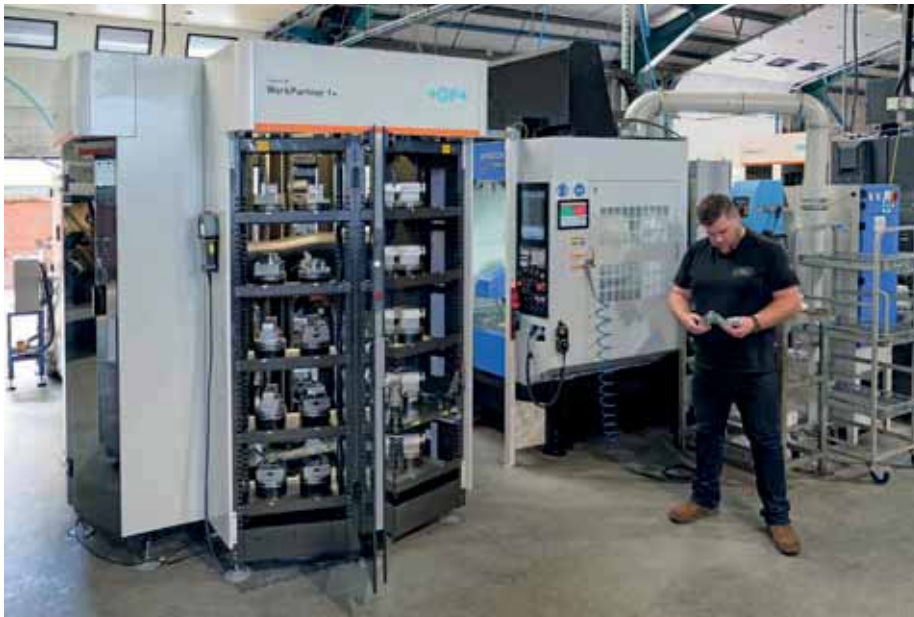
When Drury Precision Engineering was visited in June 2024, the Brother U500Xd1 / System 3R WorkPartner Plus production cell was set up to produce 18 different large and small components in left- and right-hand variants in batches of between 50 and 250.
