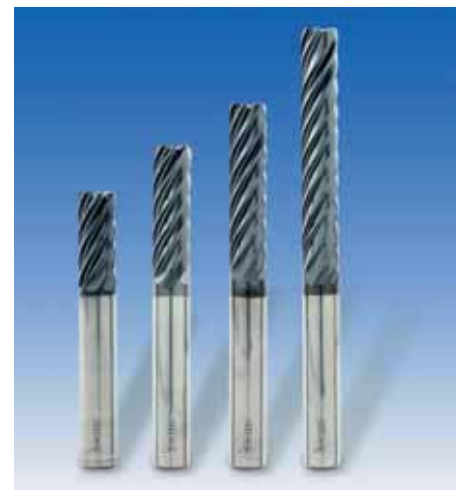
Fig. 1: The design of seven-flute solid carbide endmill for trochoidal milling features the CHATTERFREE concept to improve vibration strength.
