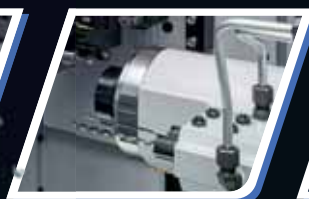
Deep hole drilling
