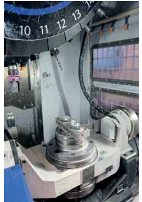
Machining area of the Brother U500Xd1 30-taper, trunnion-type, 5-axis machining centre.
