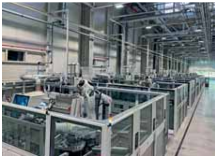
Eight automated KASTOvariospeed C 18 production circular saws process stock up to 180 mm in diameter.
