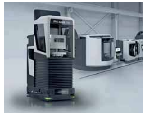
The PH-AMR 750 automated guided vehicle for autonomous pallet handling.
