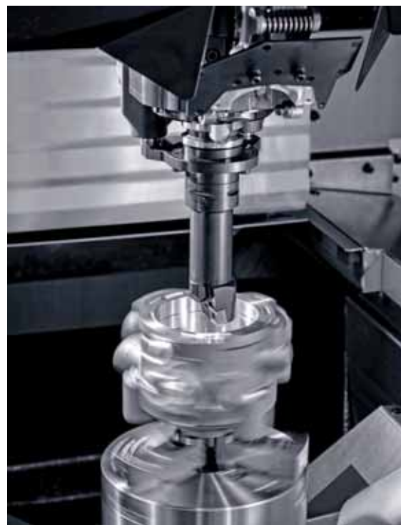
Turning operations can be carried out on the M300Xd1 using the C-axis torque table, which is mounted on a -30/+120 degree swivelling A-axis trunnion
