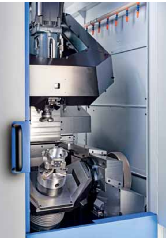
The working area of the Brother Speedio M300Xd1 30-taper, 5-axis mill-turn centre from Whitehouse Machine Tools
