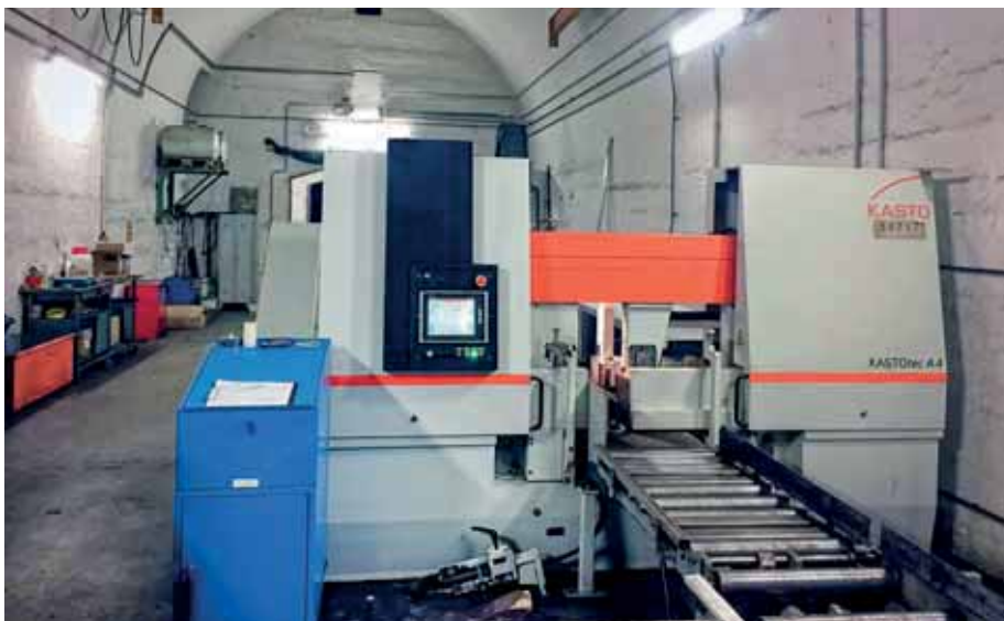
One of the KASTOtec A 4 bandsawing machines is in a historic vaulted cellar on the site.
