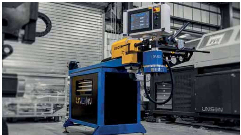
Unison EvBend 1000, manually operated, CNC-controlled tube bending machine.
