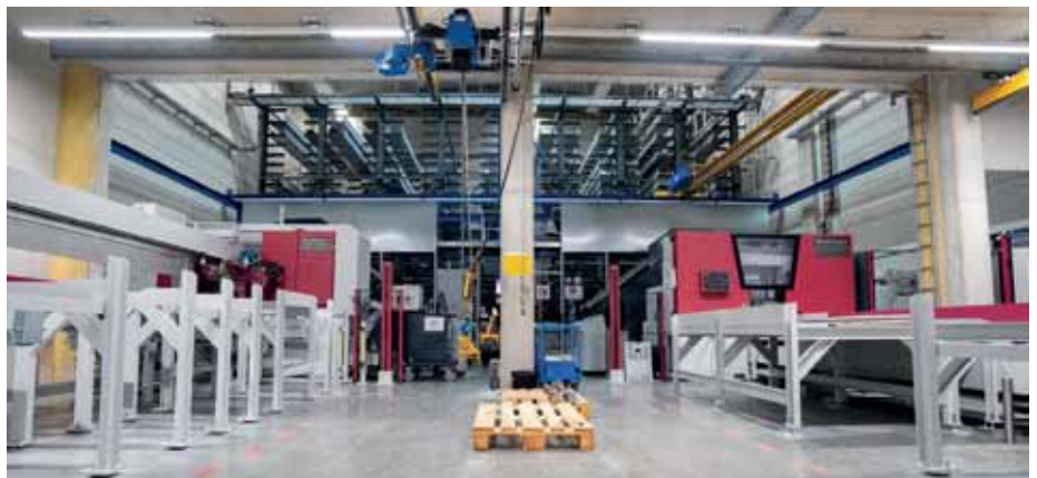
The new sawing centre consists of the HBM540A high-performance automatic band saw (left in the picture) and the HBE411A Dynamic automatic band saw. The Remmert bridge bearing can be seen in the background.
