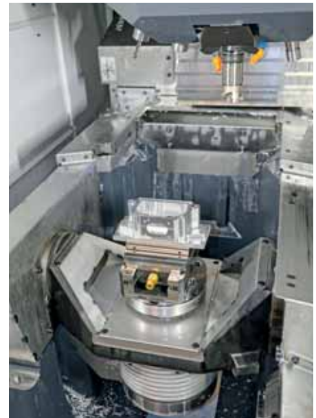
The M200X3 is one of 10 VMCs on the shop floor at R&A, working alongside eight CNC turning centres.
