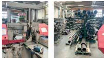
The old sawing centre consisted of two older Behringer band saws. The required sawing section had to be measured and set up manually. The material was stored in cantilever bearings and stored and retrieved by an overhead crane.
