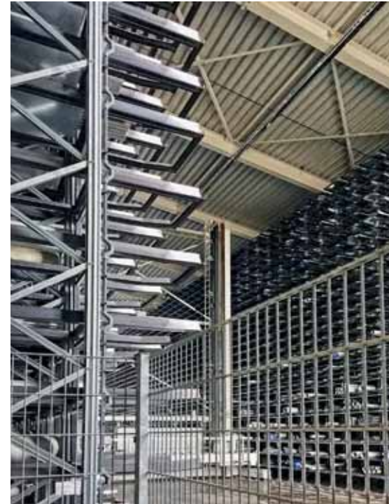
The KASTO Unicomact storage system installed at Austrian tube stockholder Karl Mertl Handelsges significantly increased storage capacity and improved safety.
