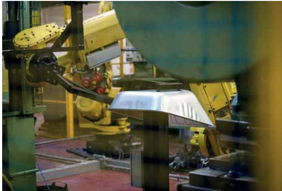
The 6-axis R-2000iA robots combine fast cycle times with high payload capabilities, making them ideal for the pick and place tasks they perform at The Walsall Wheelbarrow Company.
