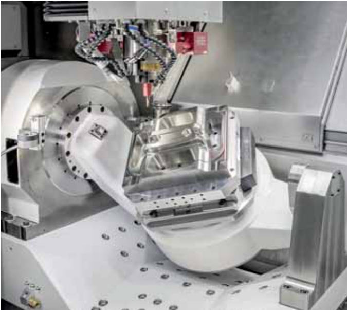
Machining area of the RPT800DSH in which, for the first time, the machine table and rotary axis bearings, in addition to the torque motors, are thermally controlled. Spindle zero point in the Z-axis is measured to sub-micron accuracy using an external, non-contact sensor to enable growth compensation.
