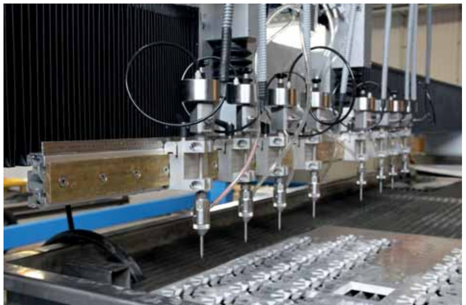
Eight high-performance abrasive nozzles strategically mounted on a beam for efficient volume production.
