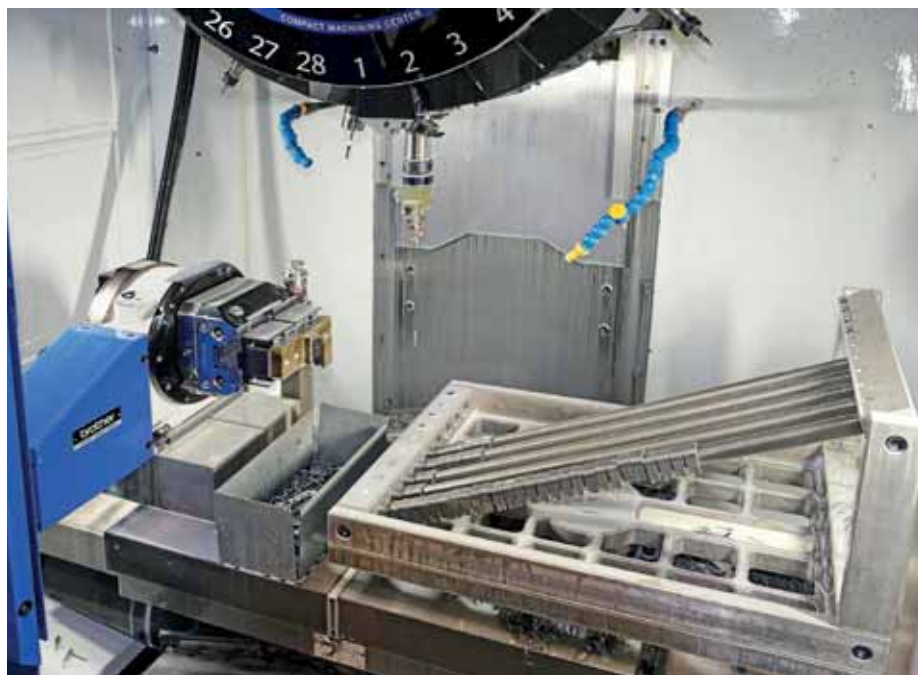
The machining area of one of the Brother Speedio S700Xd1 30-taper machining centres on the shop floor at Westley Engineering's Birmingham factory. It shows the fixture (right) with multiple inclined bars holding the brake clips, allowing hundreds of them to be presented for drilling and countersinking in one hit before the machine doors are opened again.
