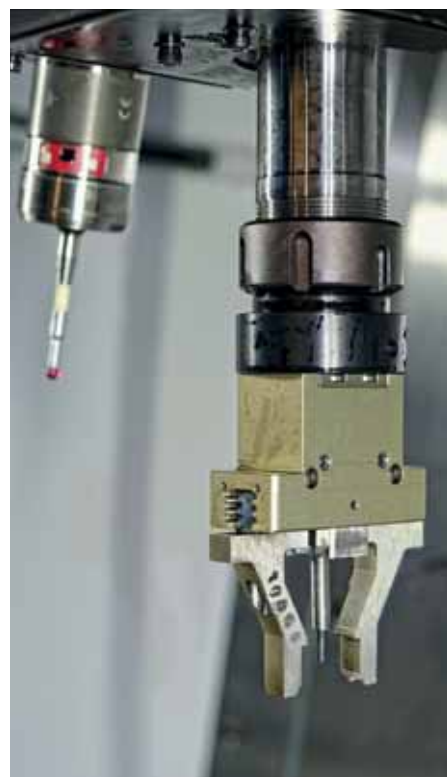
The workpiece gripper in the tool carousel of the Brother S700Xd1.
