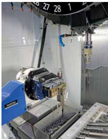
Close-up of the Schunk hydraulic vice on the rotary table, the workpiece sensor to the right of it and the coolant-actuated workpiece gripper (top right).
