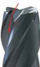
End Cutting Edge Chip Pocket Optimised geometry of the end cutting edge for excellent chip evacuation.
