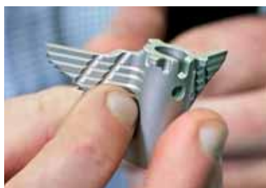
This stainless steel keel punch used in total knee replacement surgery is 90 percent machined on the Brother much faster than previously and to within 15 to 20 microns over the entire form.
