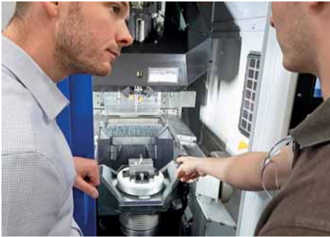
Adam Thornton (left) with one of Kirkstall's setter-operators in front of the Brother machining centre, showing the rotary torque table that allows in-cycle turning operations to be completed.
