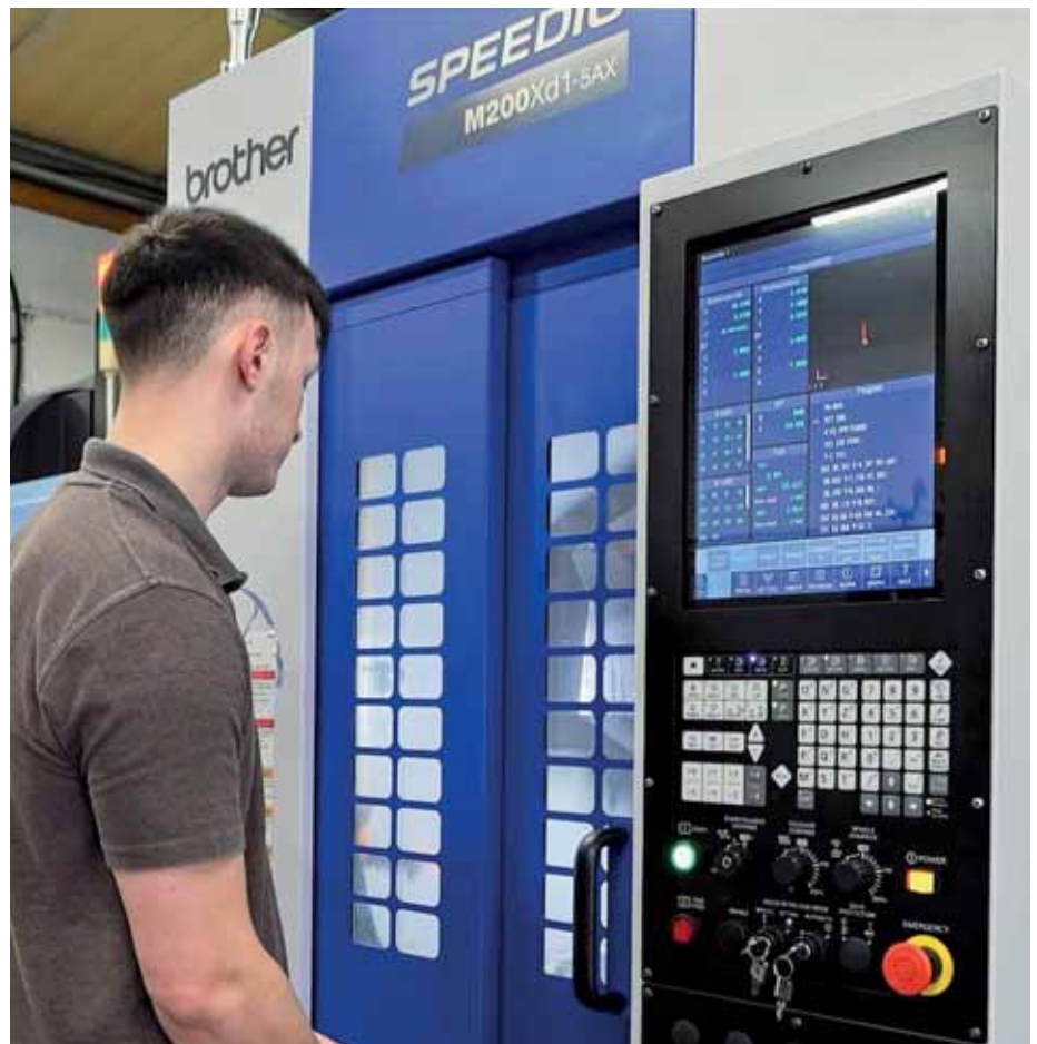
The Brother SPEEDIO M200Xd1-5AX on the shop floor at Kirkstall's Leeds facility. The high-speed, BBT30, 16,000 rpm spindle machine, normally associated with cutting aluminium and other light materials, here machines mainly stainless steel, titanium and other tough alloys.
