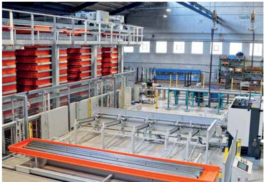
The new storage systems have improved workplace safety, since material is now transferred automatically to the saws.
