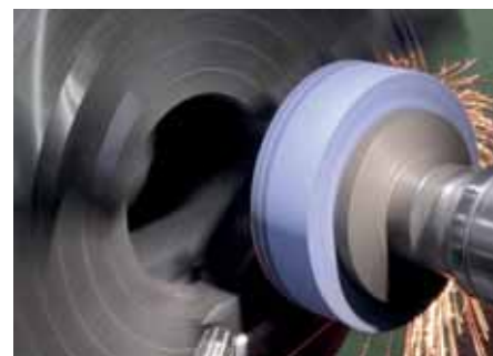
Finish grinding of the clamping jaws for the DURO-M lathe chuck.
