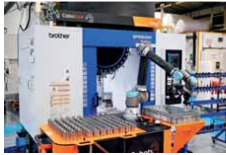
Two views of automated production of a component in the Brother Speedio cell. The cobot grippers are manufactured in-house by AML.
