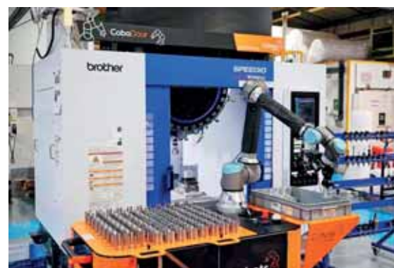
Above: Four Views of the Brother Speedio W1000Xd2 with Cobots Online component handling on the shop floor at ALM, Newton Aycliffe.
