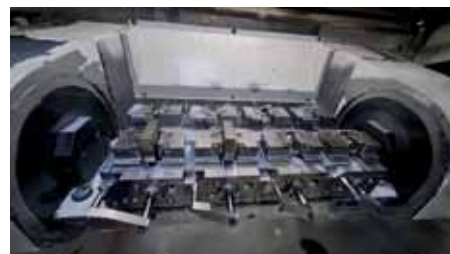
8-station clamping fixture within the automated production cell: Here, the stepped jaws are securely clamped for the machining processes.
