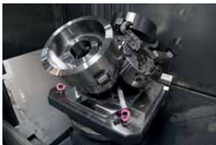
The 4-station clamping solution from RÖHM reduces idle times and enables a production process that is ten percent more productive.
