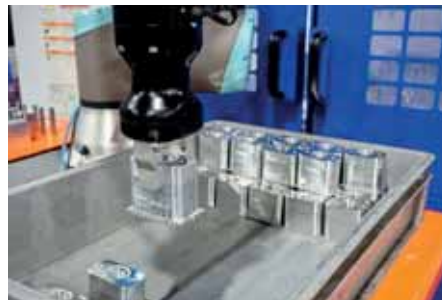
Two views of automated production of a component in the Brother Speedio cell. The cobot grippers are manufactured in-house by AML.
