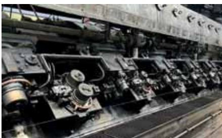
A finished block with the carbide rolling rings machined on the Lean Selection shaft.
