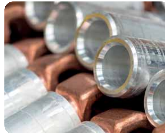
A dissimilar metal weld.
