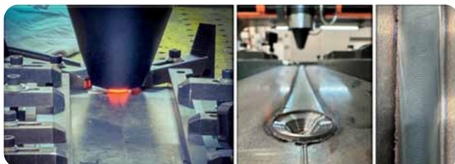
Friction stir welding of steel.
