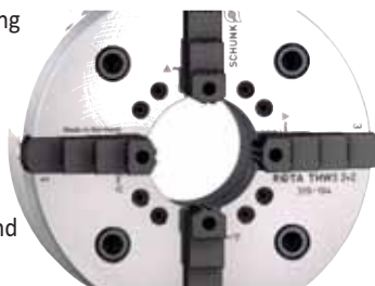
The 4-jaw lathe chuck features independent positioning of the two jaw pairs with centrally compensating workpiece clamping, allowing companies to clamp round, cubic, or geometrically irregular workpieces equally well.
