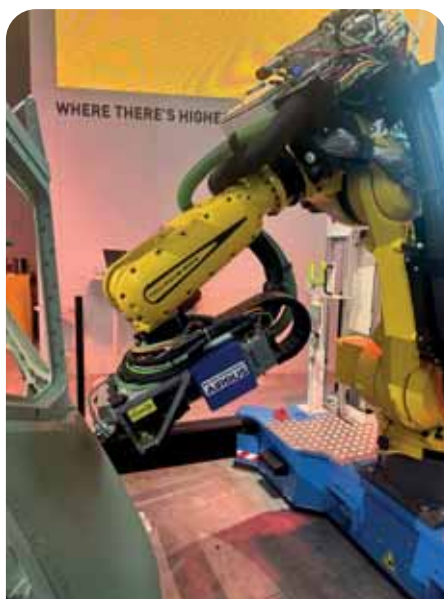
Airbus' first in-house robotic drilling cell, built with FANUC, features an M-800iA/60 robot controlled by a FANUC CNC.
