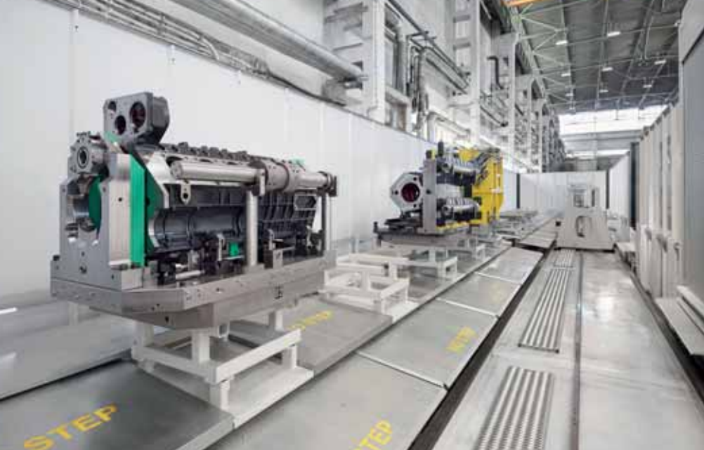
Tatra chose a pallet system as the automation solution, which initially contains twelve pallet spaces.
