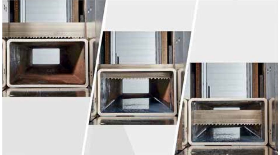
KASTOrespond continuously optimises the parameters of the sawing machine to maximise blade downfeed, according to the material cross section the blade encounters and any hard spots in the material. Left: prior to starting the cut. Centre: Without using the software. Right: With KASTOrespond switched on.
