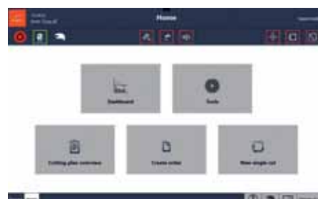
Simple Mode simplifies the display to show only essential functions and supports safe operation of the saw by novice users.
