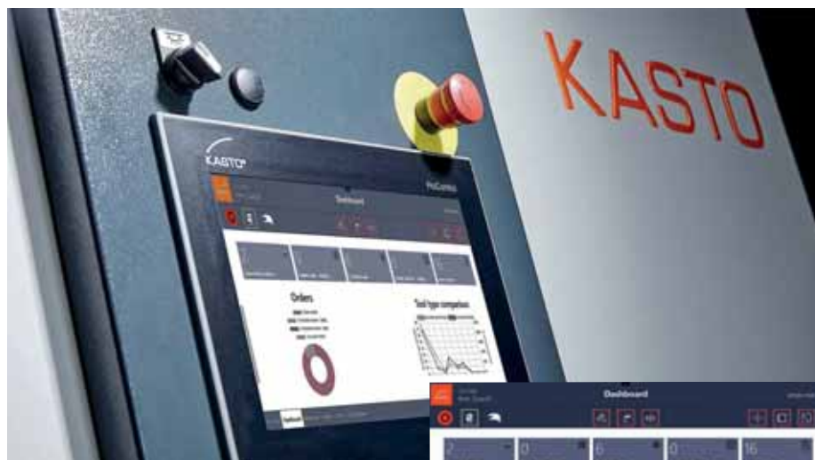
The dashboard of the new KASTO saw control provides a clear overview of machine status, job orders, runtimes and downtimes.
