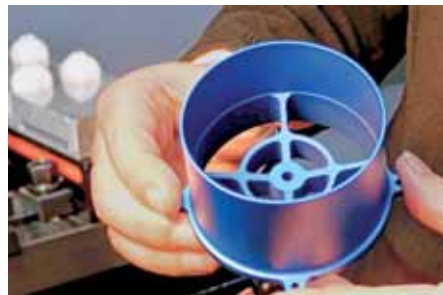
This manifold was held in a QwikLOK on just 3 mm of material prior to milling.
