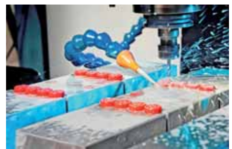
Another Chick QwikLOK being used to hold multiple round parts, this time for an RPH Parallel Lock kit.
