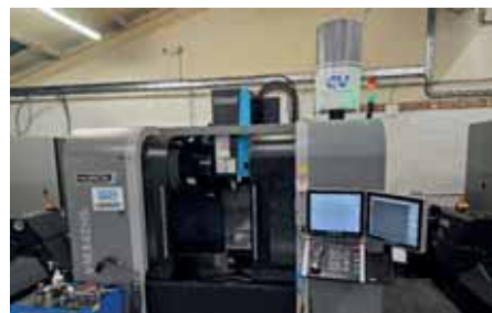
Clarion LEV installed on a Hurco VMX42HSi at CGP Engineering.
