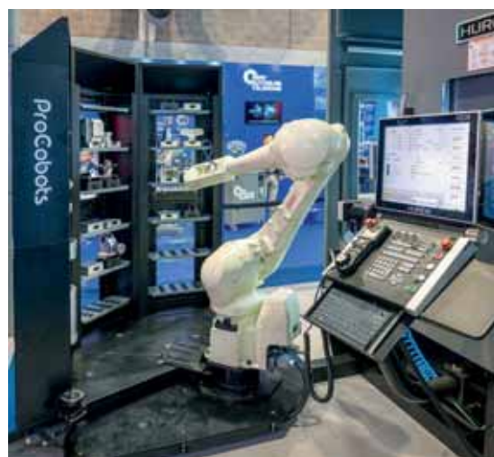
A PC25 Kawasaki 6-axis robot automation cell similar to the one that will be delivered to MK Precision later this year to automate the Hurco VMX42SRTi.
