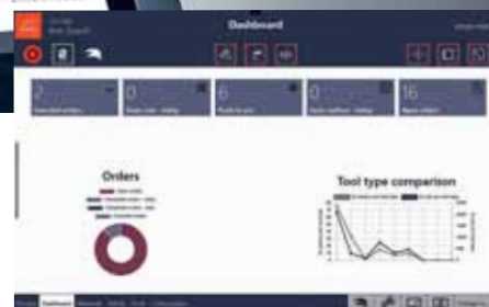
The dashboard of the new KASTO saw control provides a clear overview of machine status, job orders, runtimes and downtimes.
