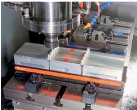
A twin-station Chick QwikLOK with machined soft jaws being used on a Hurco VMC to slot mill 10 securely-held components at a time.
