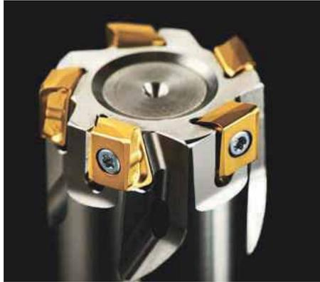
A single flat rake face on the insert improves chip disposal and provides accurate wall face step overs with a cusp height of only 8 µm when deep wall machining. Additionally, the minor cutting edge that blends smoothly into a large corner radius also provides a benefit by providing the ability to achieve good component surface finishes. The top face geometry combines the minor cutting edge and a relief angle that makes ramping possible.
