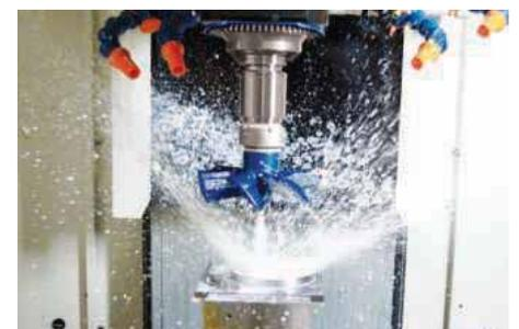
Fan means chips and coolant can be quickly and easily removed without any interruption to production. This maximises productivity and prevents unpleasant costly delays."
