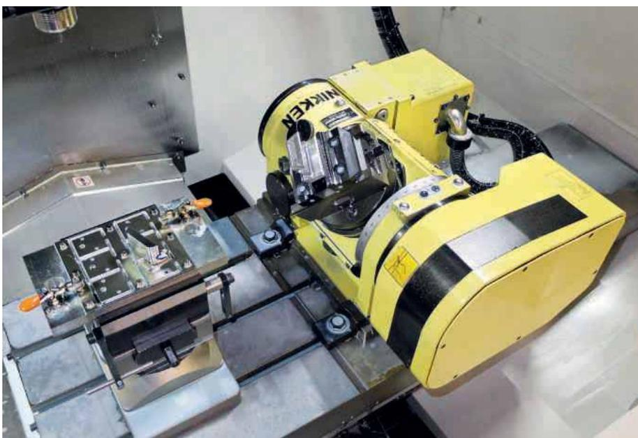
the Suffolk subcontractor's capabilities. Six components are required, half of which are suited to 3-axis metalcutting while the others benefit from five-face machining in two operations using 3+2-axis cycles, as otherwise they would need eight setups on a 3-axis machine.
