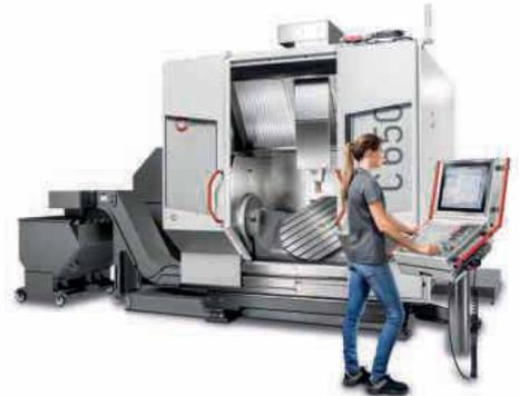
Standard CNC system is Heidenhain's TNC 640, which offers the full programming capability of this proven, high-end control. The GUI has a large, full colour, 19" TFT flat panel monitor and the control can be swivelled to the magazine loading station so that the operator can enter tool data directly into the control.
