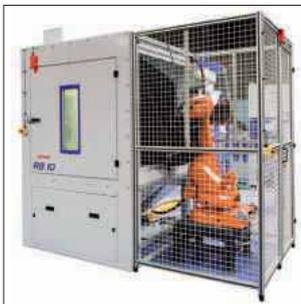
Guyson International's advanced robotic blast systems deliver benefits for manufacturers of precision components with demanding surface engineering topography requirements and any subsequent validation issues, typically medical implants and aerospace turbine blades.
