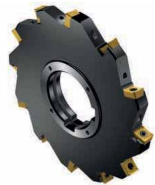
Ease-of-use is a further requirement of machine shops the world over. For this reason, CoroMill 331 makes use of spring-loaded cassettes with serrations that provide security and easy setting for the desired width. Moreover, a pin-controlled adjustment range enables manufacturers to set the cutter with high accuracy for precise groove dimensions.
