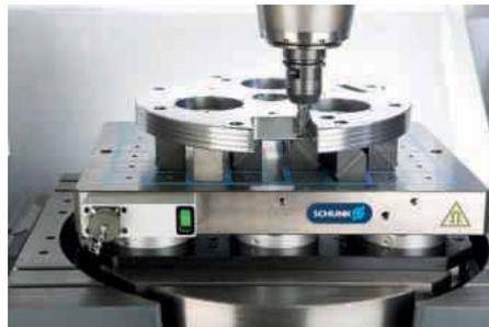
demanding applications. Due to the conical fitting, the clamping pins can also be joined into the modules eccentrically, making this process incredibly easy. The actual clamping is done via spring force without any external energy supply; it is form-fit and self-locking. The workpieces remain safely clamped in case of a sudden pressure drop in the air system. A pneumatic system pressure of six bar is sufficient to open the clamping modules.
