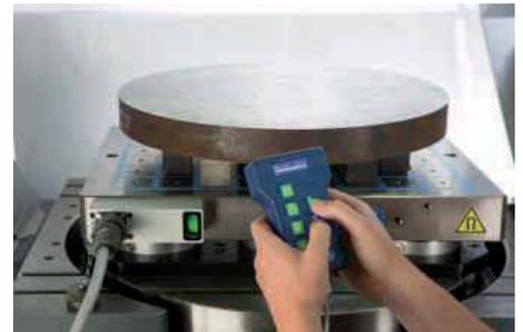
To ensure process reliability in automated applications, it is possible to monitor each individual magnetic chuck. To do this, the individual clamping state is transmitted via a PLC interface to the system control. The SCHUNK MAGNOS KEH plus control unit is completed by the handheld remote SCHUNK MAGNOS HABE-S plus that is also modular. This allows control of the individual magnetic chucks and the individual 16-step holding force regulation process.
