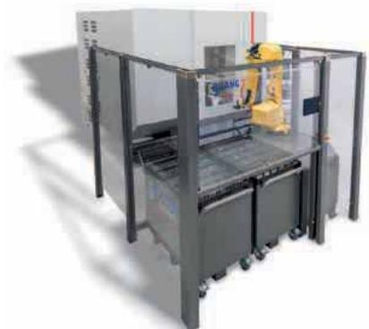
An intuitive, easy-to-operate touch panel enables easy control of the automated system and, as external access to the trolley is possible, production remains seamless as machining cycles do not need to be interrupted. Control of the zero-point clamping system can be performed either pneumatically through the machine tool or mechanically through the system's robot.
